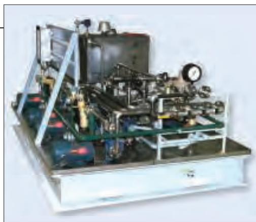
FIGURE 2. Shown here is an example of a compact lubrication skid for a shop test-stand facility
